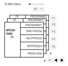
15 programs can be entered here which have been created with the ECL interpreter and have been uploaded to the summator via the data interface.
