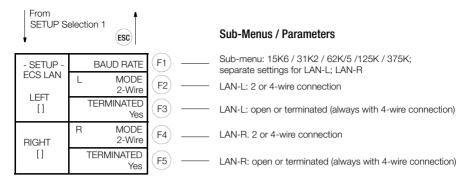
LAN-L: Settings for LAN left (terminals 49 through 52) LAN-R: Settings for LAN right (terminals 53 through 56)
