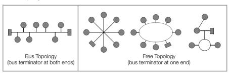
If a bus structure is used, the components are connected in parallel, one after the other. A bus terminating resistor must be used at each end. Branch lines may not exceed a length of 3 meters. Only one bus terminator is required with free topologies, but transmission distances are limited in this case.
