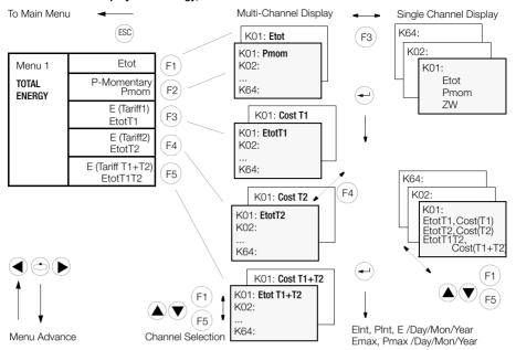
• Multi-Channel Display (all channels with only 1 measurement value)
